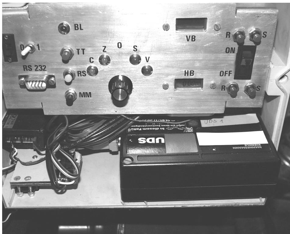
Figure 2: Accident-data recorder UDS (“black box“) installed in the data acquisition box, mounted on the right-hand-side of the motorcycle.
