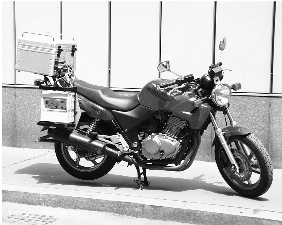
Figure 1: Instrumented motorcycle Honda CB500 as used in the experiments. 2.1 Measurement equipment
