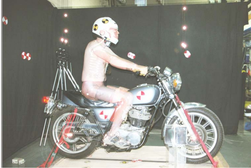
Figure 2. Illustration of comparison of human subject position relative to MATD ISO13232 position.
