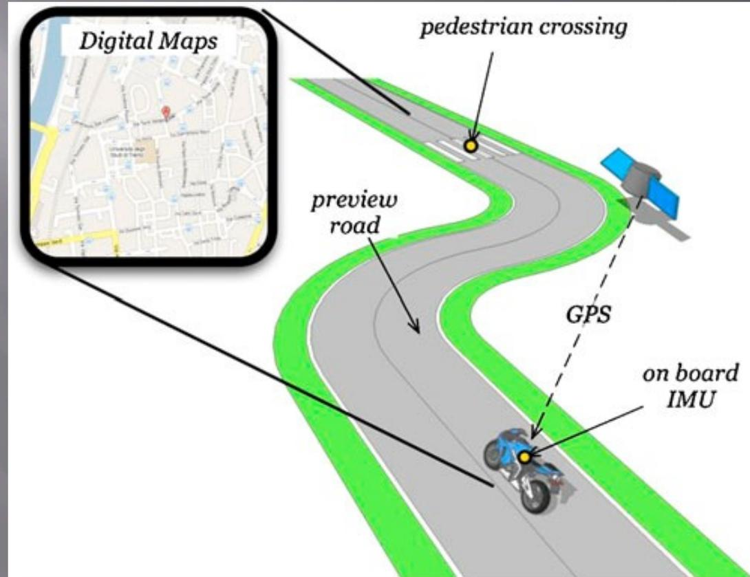
Typical scenario and main sensors used in the curve warning function (Biral, et al. An intelligent curve warning system for powered two wheel vehicles, 2010)
