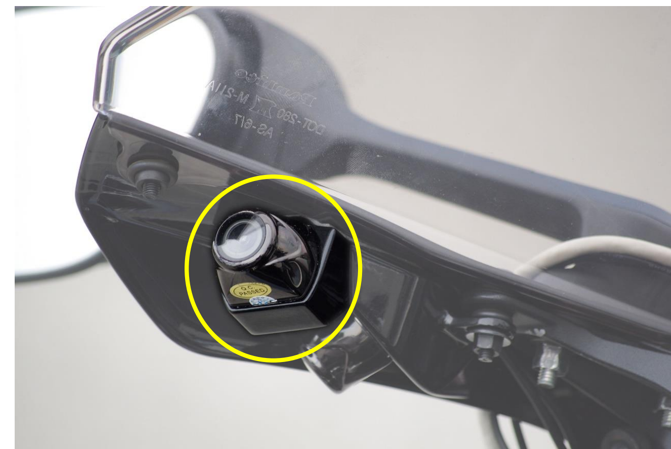
Small camera installed to monitor rider's face
