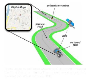
Typical scenario and main sensors used in the curve warning function. Source: (Biral, et al. An intelligent curve warning system for powered two wheel vehicles, 2010)
