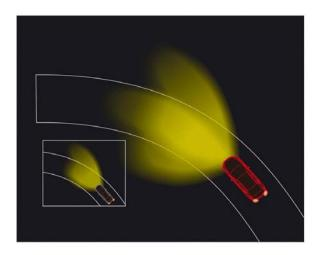
2014 Mazda 6 Adaptive Front-lighting System (AFS) photo Source: http://www.bing.com/images/search?q=Adaptive+Front+Li ghting+System+(AFS)&FORM=HDRSC2#view=detail&id =316096632B2331CA36737DA9BF712B178935F1B8&sel ectedIndex=0
