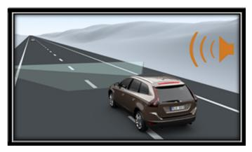
Volvo's lane departure warning system scans the road ahead to identify lane markings. Source: <u>http://carbuzzard.com/2011/11/extra-eyes-automotive-</u>lane-departure-warningkeeping-technologies/
