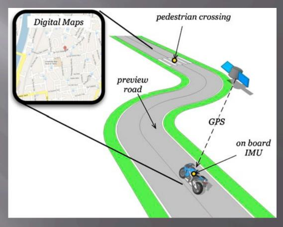
Typical scenario and main sensors used in the curve warning function (Biral, et al. An intelligent curve warning system for powered two wheel vehicles, 2010)
