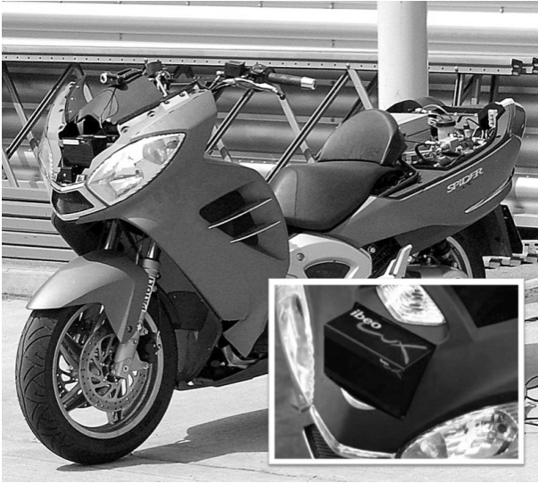
Figure 1: Prototype vehicle of the PISa project equipped with AB system (in the box: laser scanner mounted in the front fairing).
