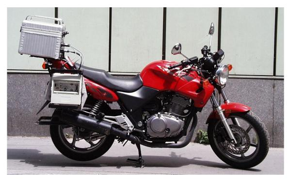
Figure 1: Instrumented motorcycle Honda CB500 as used in the experiments.
