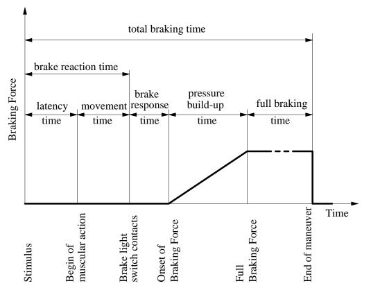
Figure 4: Sequence of events in the course of a braking maneuver.
