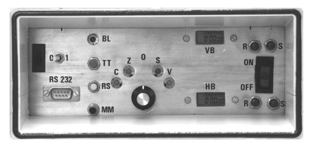
Figure 2: Front panel of the data acquisition box with digital timers VB and HB for front-wheel and rear-wheel brake operation, respectively.
