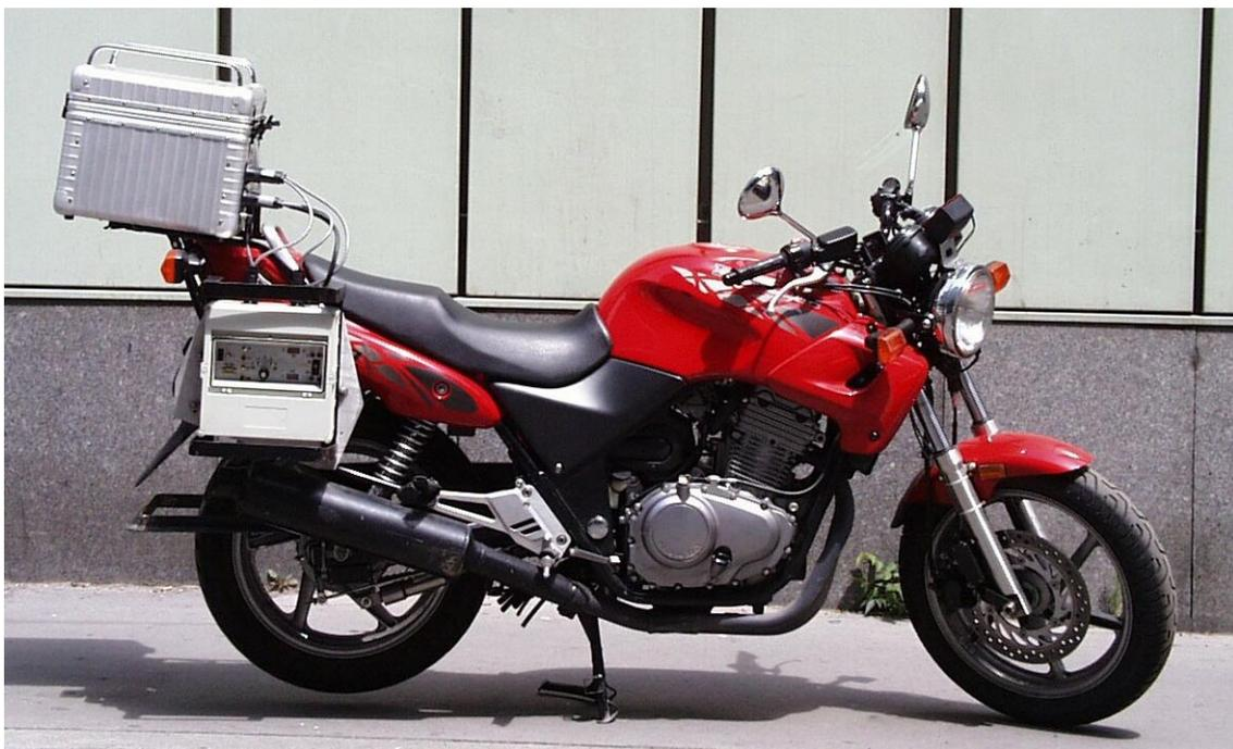
Figure 1: Instrumented motorcycle Honda CB500 as used in the experiments.
