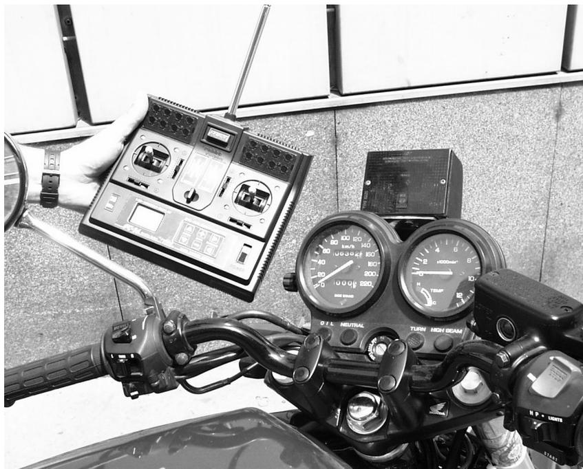
Figure 3: Signal lamp mounted next to the speedometer. Remote control to trigger signal lamp.
