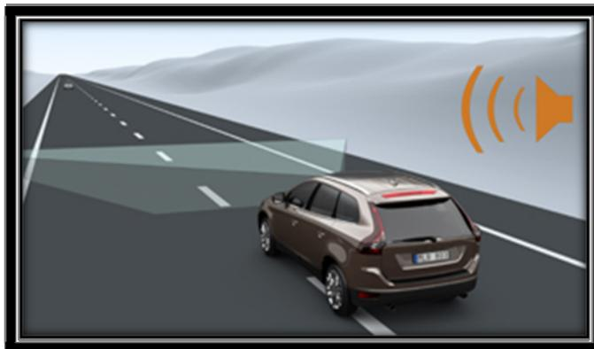
Volvo's lane departure warning system scans the road ahead to identify lane markings.
