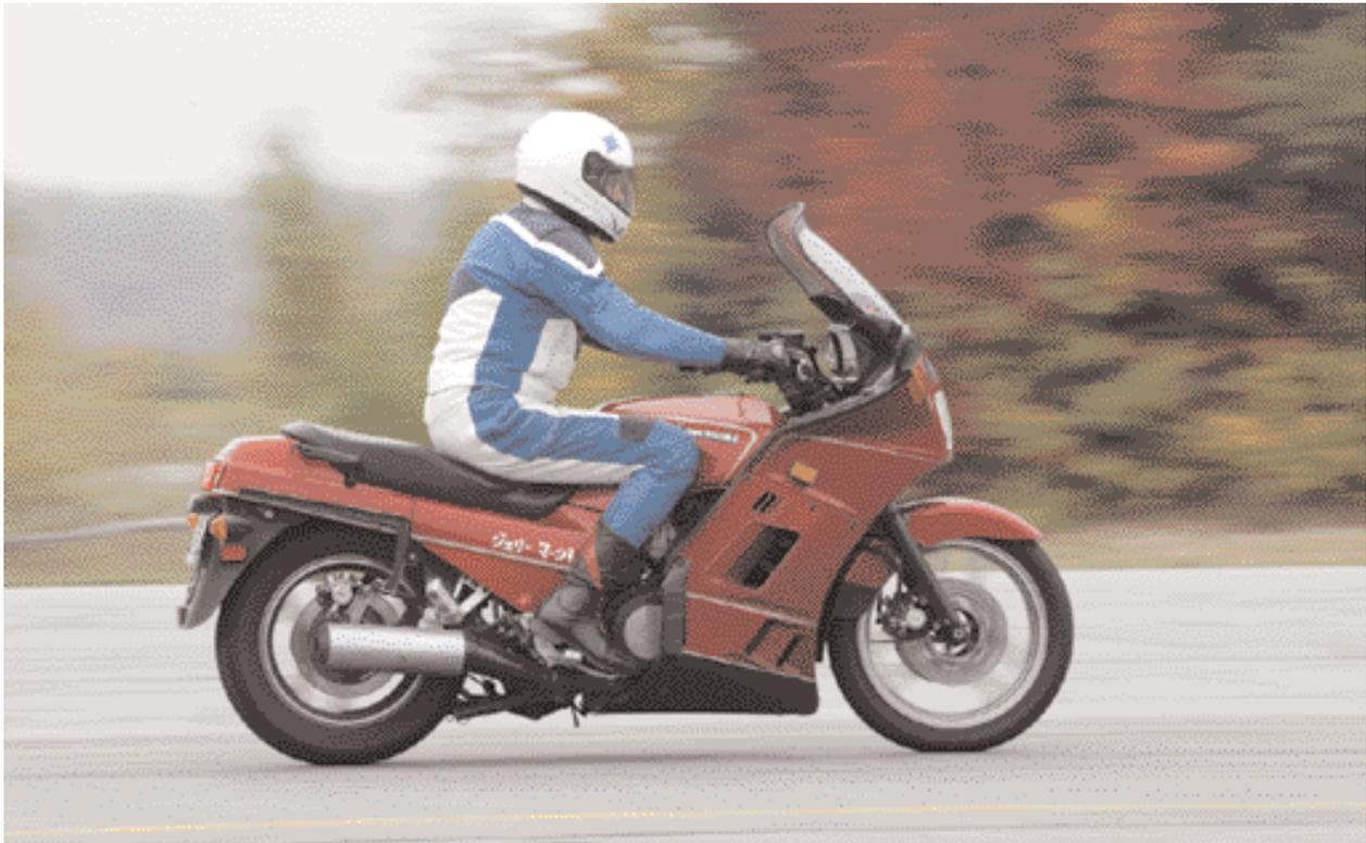
On the great majority of current motorcycles the brake for the front wheel and the brake for the rear wheel are activated by separate controls. The front brake is activated by the lever on the right handlebar and controlled by the rider's hand. The rear brake is activated by a pedal mounted close to the right footpeg and is controlled by foot.
